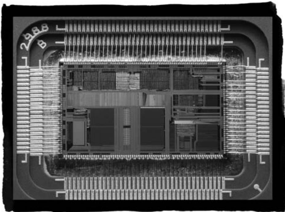
**Photo #2: A Microchip with the Cover Removed**
